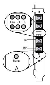
Figure 5. Location of the LEDs (dual link)
